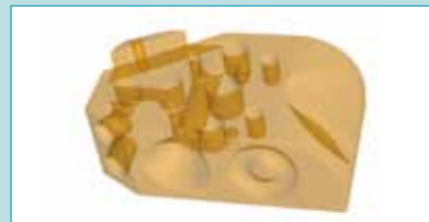
Volume model of the component in semi-transparent display. The internal structures are visible
