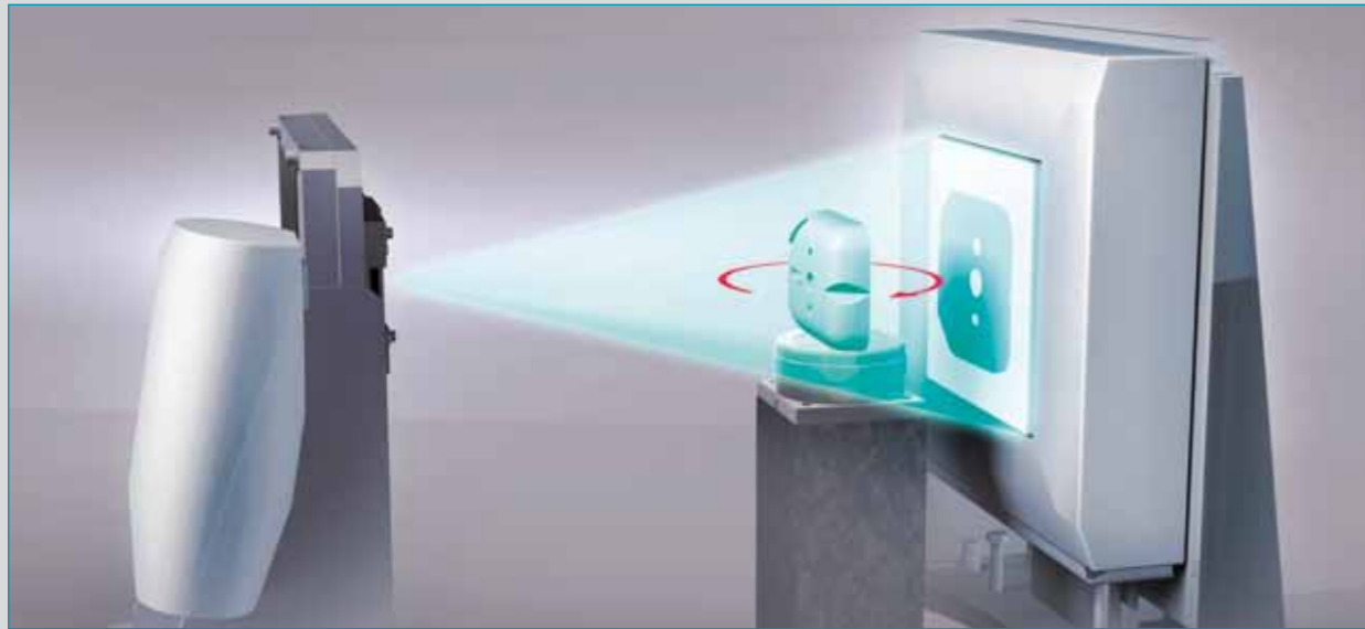
Operating principle of the exaCT.M: The component is rotated in the path of the X-ray beam and a three-dimensional model is reconstructed from a number of two-dimensional projections.
