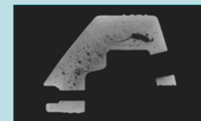
The virtual 2D section shows porosity in the component
